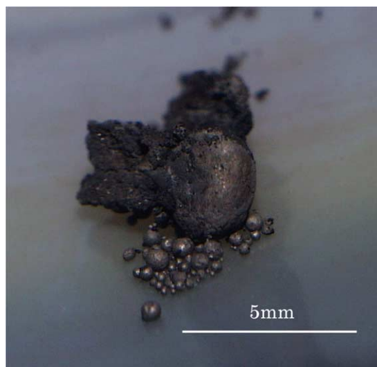
Fig. 7. Residual HM alloy obtained in RUN 2.
