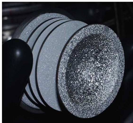
Fig. 4. Cadmium deposit on the baffle plates of the condenser rid.
